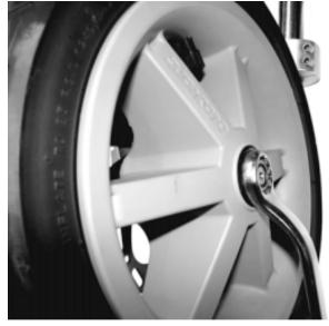
Fit your wheel to the fork and secure with 12mm axle nut. Rotate the wheel on the axle to make sure that the rotor screws don't rub on the bracket.
