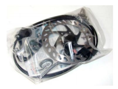
Note: This brake kit will only fit the current forged alloy front fork (released Feb 2007)
