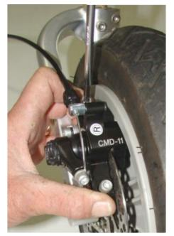
Align the calliper so the rotor is centered in the slot of the alloy casting and secure the alignment screws.
