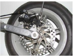
Remove the calliper mounting screws from the calliper mounting block. Loosen the brake pads on the calliper by rotating the adjusters either side and align the mounting block with the holes on the fork.
