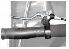
Parking Brake: The brake also includes a locking system to be used as a park brake.
