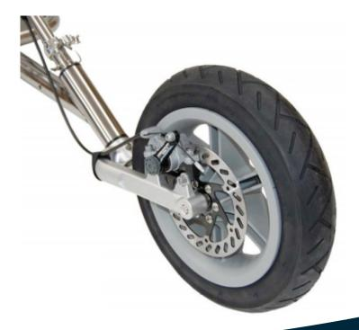
The Blokart Disc Brake is a piece of high precision equipment with fine tolerance. Any sand or grit from beach sailing may affect its performance.
