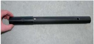
1. Slide a sleeve over the rear axle stub on the shadow ensuring the sleeve hole locates with the existing spring button.
