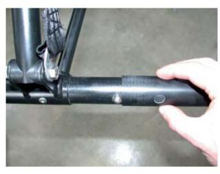
2.Slide the other sleeve over the shortened axle that will go into the right side of the SS blokart chassis.
