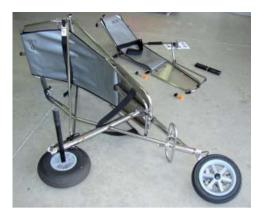
5. Lift shadow over blokart and insert rear axle stub of the shadow into the rear axle tube of the blokart chassis. Do not locate the spring button into the chassis hole yet.
