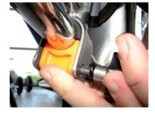
9. Undo the shadow foot bar star knob and refasten with plastic clamp around the blokart foot bar.
