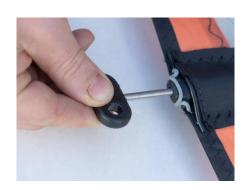
**Notes:** Do not overtighten the Adjusters as this may damage the batten pocket. The best performance is achieved with soft tension. Reduce tension on the batten by turning the screw in anti-clockwise direction.
