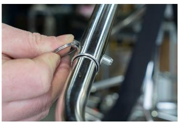
8. Attach the safety bar to the Blokart mast base by removing the left star knob, sliding the safety bar over the mast base stud and the re-tightening the star knob and attaching the safety clip.
