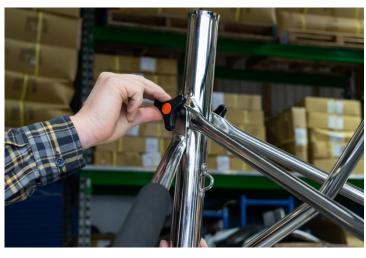
9. Swing down the small arm on the safety bar and attach to the Shadow chassis with the small star knob. Gently roll the chassis flat again
